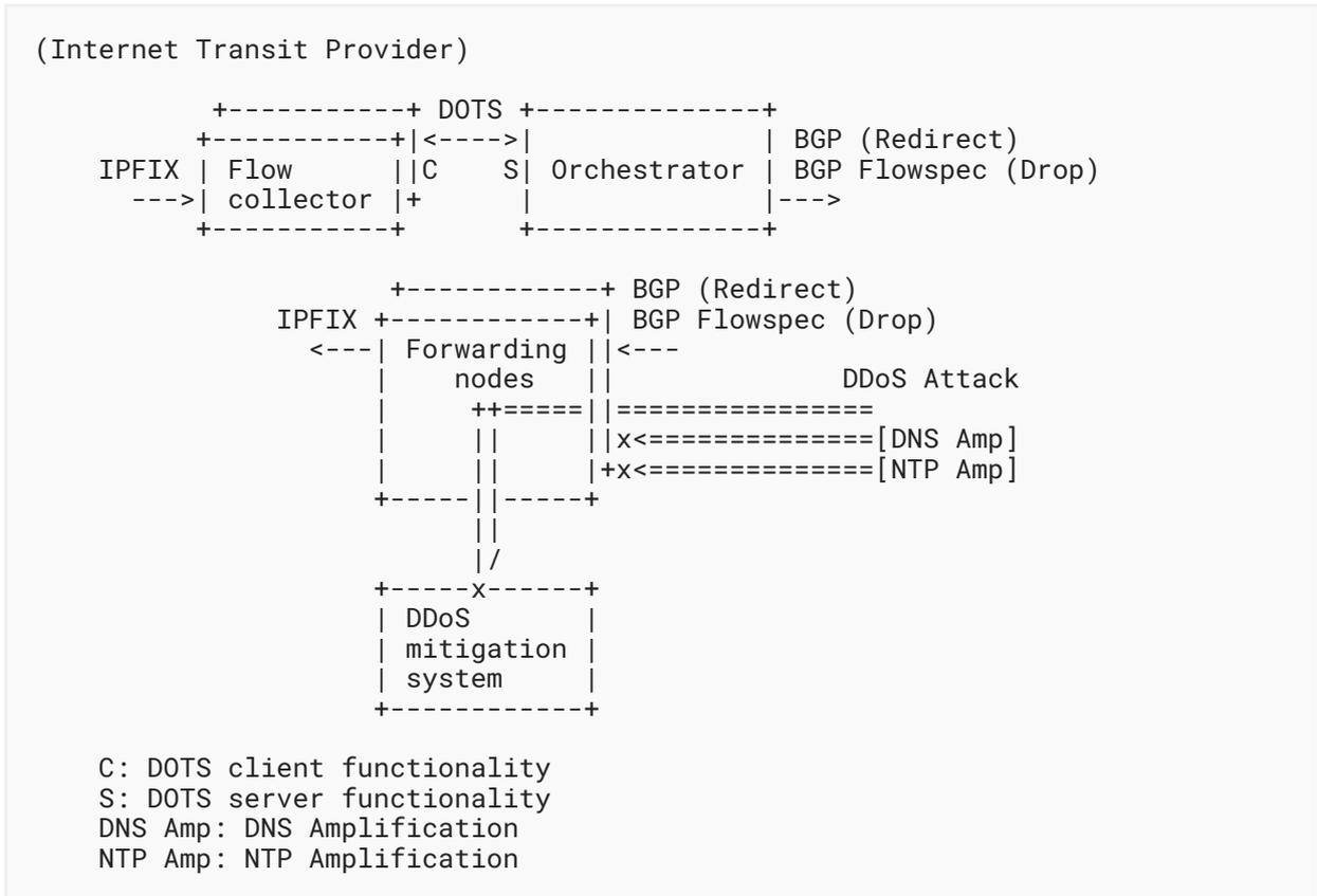
Figure 10: Selecting Mitigation Technique Based on Attack Type
