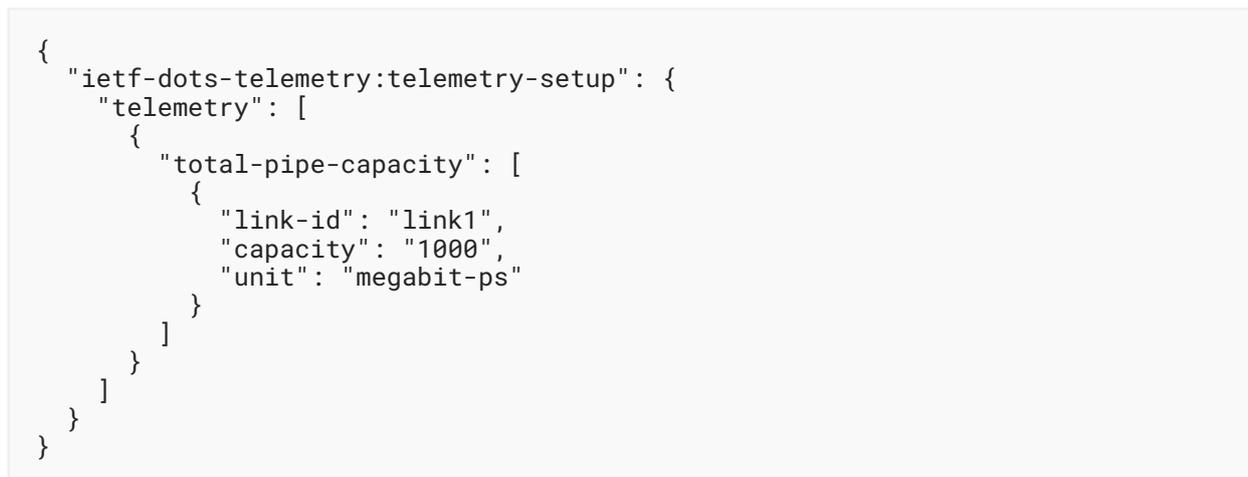
Figure 14: Example of Message Body with Total Pipe Capacity
